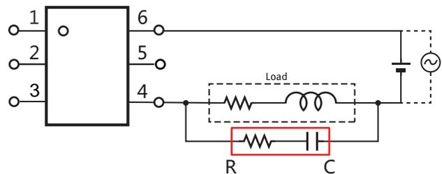
When adding diodes, buffer circuits (C-R), and other protections, they need to be installed near the MOS RELAY to be effective.
