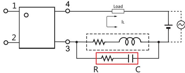
When adding diodes, buffer circuits (C-R), and other protections, they need to be installed near the MOS RELAY to be effective. Adding protection elements may result in a slow reset time, so adjust them according to the actual situation before use.
