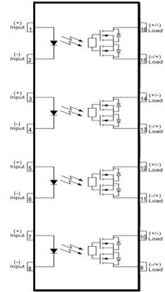
LED forward current must be more than 5mA , at  $I(\text{MIN})$  ,and less than 30mA , at  $I(\text{MAX})$ .
