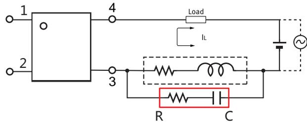
When adding diodes, buffer circuits (C-R), and other protections, they need to be installed near the MOS RELAY to be effective. Adding protection elements may result in a slow reset time, so adjust them according to the actual situation before use.
