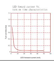
LED foward current Vs. turn off time characteristics (sm off time ŝ 40 20 30 50 60 LED forward current (mA)
