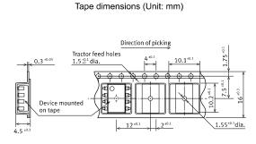
Dimensions of paper tape reel (Unit: mm)
